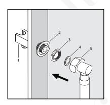
3. Install hand shower cradle (1) to the shower panel by installing the rubber washer (2) and the locking nut (3) and attach white plastic hose tube connector (5) with PVC tubing to complete the connection. (**NOTE:** Make sure the silicon gasket (4) is seated properly inside the connector.)
