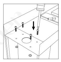
1. Remove top cover. Attach the top panel to the main body with the supplied nuts and bolts. Run the water supply hoses through the hole on the top panel.
