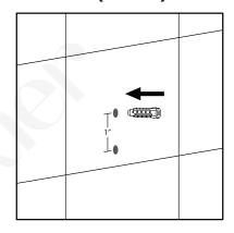
5. Using a drill with a tile bit, drill the hole slowly into the tile. Do not drill into any piping or wiring in the wall. Insert the anchors into the wall.
