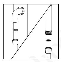
8. Once the shower panel has been tested for functions and leaks. Hang the unit on the wall to complete the installation. Due to the limited space behind the shower panel, do not bend the hoses. Any restrictions in the water supply hoses will greatly reduce the performance of the shower panel. After the shower panel is set properly on the wall, apply silicon sealant on both sides of the shower panel to prevent the unit from moving.
