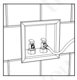
7. Apply thread sealant tape to the threading on the shut-off valves before connect both hot and cold water supply hoses to the valves.
