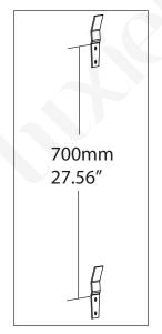
4. Lift the panel to determine the proper height and placement. It is recommened to aim the top horizontal body jet to the chest area for optimal showering experience. Mark the positions of the 2 brackets on the wall and set a side the panel.
