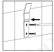
6. Secure the mounting brackets to the wall with the screws.
